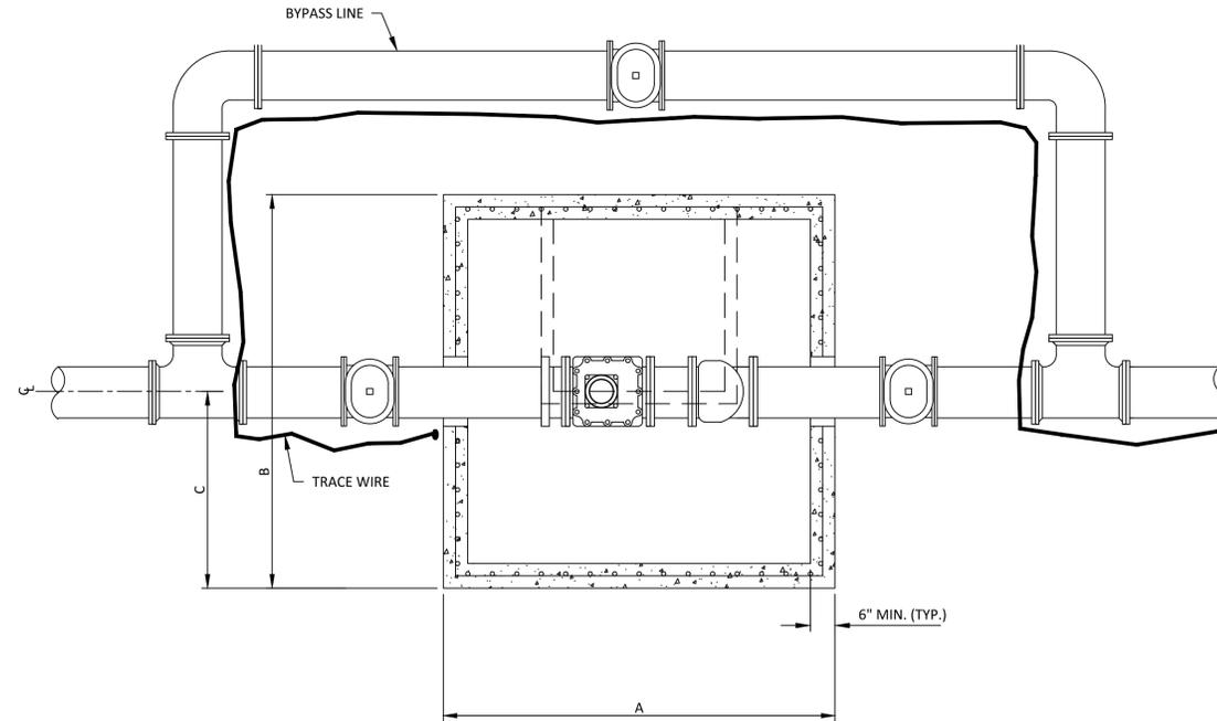
TYPE A METER VAULT (SECTION TOP VIEW)
