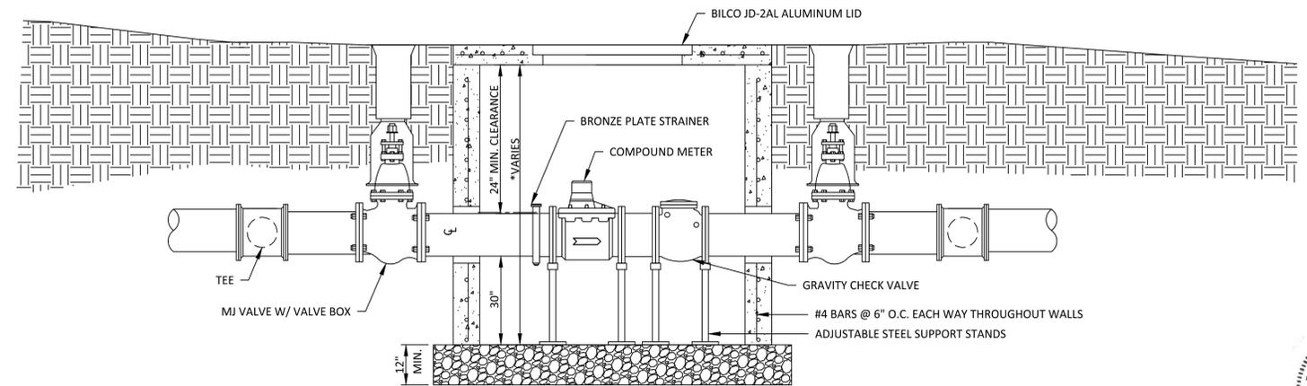
TYPE A METER VAULT (SECTION VIEW)
