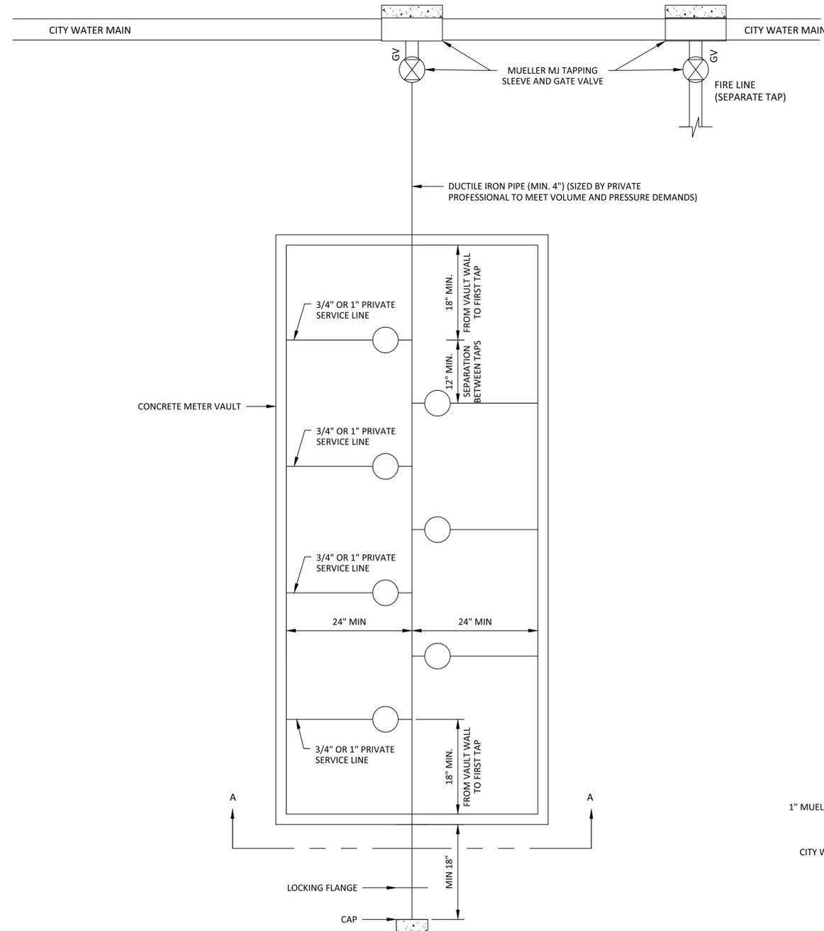
DOMESTIC WATER SERVICE - METER VAULT DETAIL
